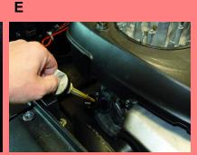
Engine is running but machine is not moving A Check setting of freewheel lever
