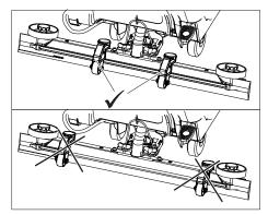
Check if the height adjustment is mounted on the inside of the vacuum bar.
