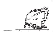
➔ Fix the ramp on the pallet with nails.
