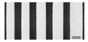
The test institute uses for the laboratory test dyed panels which are blasted with the rotary nozzle. Then the efficiency of the cleaning jet is determined based on the width of the cleaning track. The illustration on the left is an example of a tested Kärcher device compared to the results of competitor devices.
