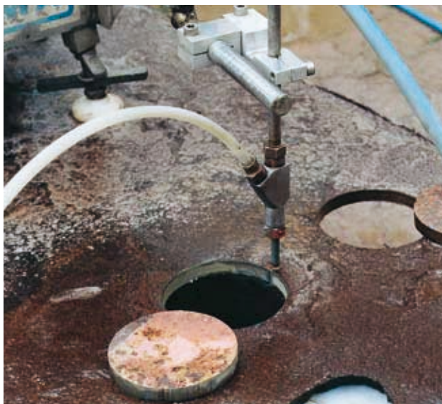
Cutting circular openings in steel plates
