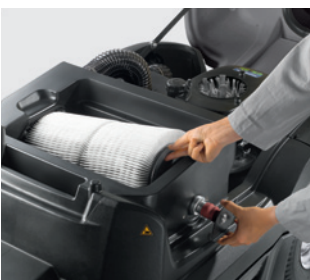
Easy maintenance Easy filter replacement.
