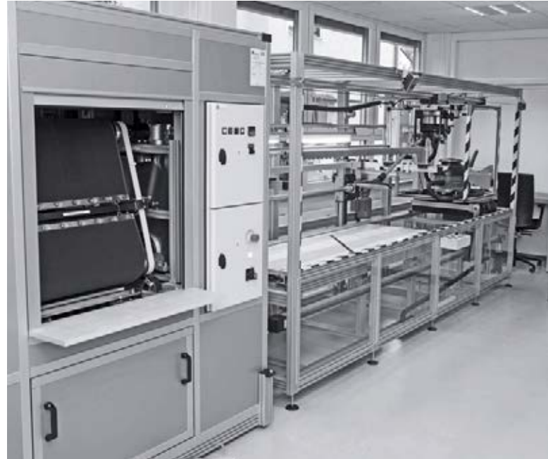
In the ErP laboratory for dry vacuum cleaners, energy use and dust intake can be measured during the cleaning of different surfaces.
