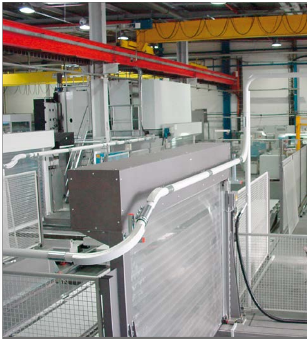
● Suction point with swivel arm and pipeline
