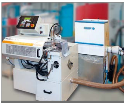
Dust remover on saws
