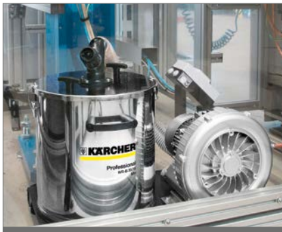
IVR-B 30/15 Me integrated into robot cell
