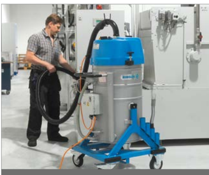
Exchange of cooling lubricants
