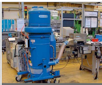
Integrated dust remover in production lines
