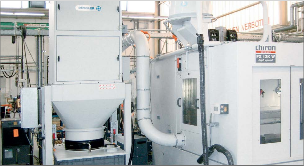
● Vacuum solution for capturing plastic chips: Ringler Kärcher Group RE 201 dust remover with FZ 12 Chiron machining centre, automatic wet/dry switch, handheld suction hose and filling level monitoring
