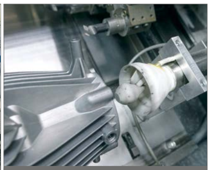
3D-printed nozzle for special vacuum functions
