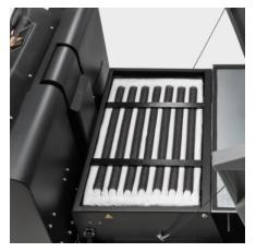
Large-area pocket filter with vibration motor
