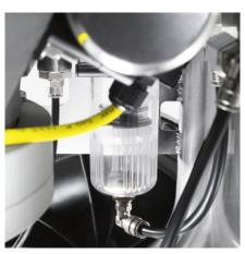
With integrated oil and water separator
