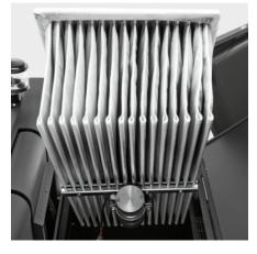
Large-area pocket filter with vibration motor
