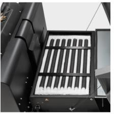
Large-area pocket filter with vibration motor
