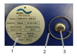
A plaque with the technical data and a fastening wire are supplied with every bursting disc. The plaque must be secured to the bursting disc bracket using fastening wire. The torque stated on the plaque for the respective bursting disc must be strictly adhered to when fitting the replacement bursting disc.
