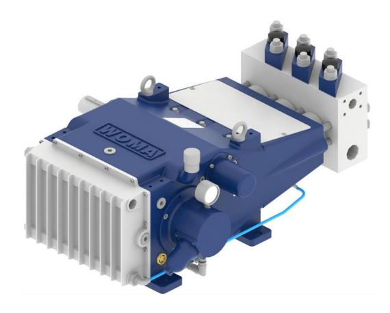
The high-pressure plunger pumps of the 2-series with operating pressures up to 750 bar and flow rates up to approx. 224 l/min, are ideal for the cleaning of pipes and tube bundles, vessels and containers. Variant V of the 2-series has been specially developed for applications with elevated inlet pressure.
