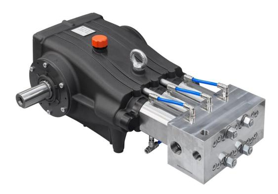
The high-pressure plunger pump of the Y series is particularly compact. Because of its small dimensions and low weight, it can be installed very well in devices with a small base frame. The pump is available with drive shaft installed right and left. With operating pressures up to 1,000 bar, this type is suitable for various cleaning tasks, e.g. in the chemical industry, in the oil and gas industry, but also in the field of ship cleaning.
