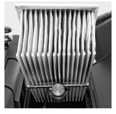
Large-area pocket filter with vibration motor
