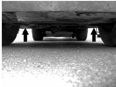
Intake point for the jack (rear wheels)
