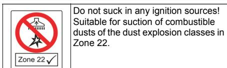
Do not suck in any ignition sources! Suitable for suction of combustible dusts of the dust explosion classes in Zone 22.
