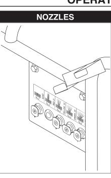
The four color-coded quick connect nozzles provide a wide array of spray widths from 15° to 40° and are easily accessible when placed in the convenient rubber nozzle holder, which is provided on the front of the machine.
