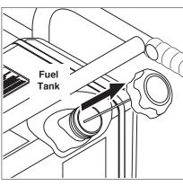
**STEP 1:** Check engine oil level. Oil level should be level with the bottom of the oil filler neck. Be sure the machine is level when checking the oil level. (Refer to the engine's operating manual included with machine.) We recommend that the oil be changed after the first 5 hours of use, then once every 50 hours. **Note:** Improper oil levels will cause low oil sensor to shut off engine. **IMPORTANT! Do not run engine with high or low oil levels as this will cause engine damage.**
