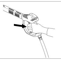
**STEP 4:** Trigger the spray gun to eliminate trapped air then wait for a steady flow of water to emerge from the spray nozzle.
