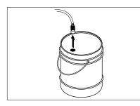
**STEP 1:** Remove detergent suction tube from container and insert into one gallon of fresh water. For low pressure connect the black detergent nozzle. Pull trigger on spray gun and siphon water for one minute.
