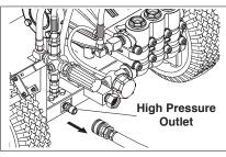
**STEP 5:** Disconnect the high pressure hose from high pressure outlet.
