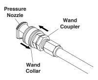
**STEP 6:** Pull the spring-loaded collar of the wand coupler back to insert your choice of pressure nozzle. Release the coupler collar and push the nozzle until the collar clicks. Pull the nozzle to make sure it is seated properly.
