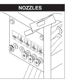
The four color-coded quick connect nozzles provide a wide array of spray widths from  $15^{\circ}$  to  $40^{\circ}$ and are easily accessible when placed in the convenient rubber nozzle holder, which is provided on the front of the machine.
