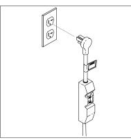
**STEP 1:** Connect machine to adequate power source. Push reset button on GFCI if equipped.
