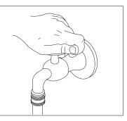
**STEP 2:** Before installing nozzle, turn on water supply and run machine allowing water to flush through the system until clear.
