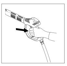
**STEP 2:** Trigger the spray gun to eliminate trapped air then wait for a steady flow of water to emerge from the spray wand. Then install nozzle.
