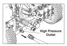
**STEP 5:** Disconnect the high pressure hose from high pressure outlet.
