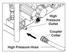
**STEP 3:** Connect the high pressure hose to the high pressure outlet. Push coupler collar forward until secure.
