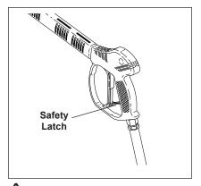
WARNING! Never replace nozzles without engaging the safety latch on the spray gun trigger.
