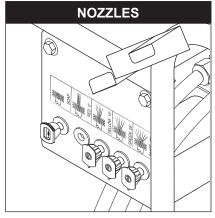
The four color-coded quick connect nozzles provide a wide array of spray widths from 15° to 40° and are easily accessible when placed in the convenient rubber nozzle holder, which is provided on the front of the machine.
