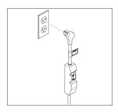
**STEP 1:** Connect machine to adequate power source. Push reset button on GFCI if equipped.
