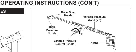
Selection of high or low pressure is accompanied by turning the handle. **Note:** High pressure nozzle must be inserted at end of wand to obtain high pressure. To apply soap read operator's manual.
