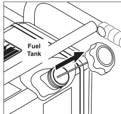
**STEP 2:** Fill the fuel tank with the appropriate fuel (unleaded gasoline or diesel as noted on the tank). Do not use leaded gasoline.
