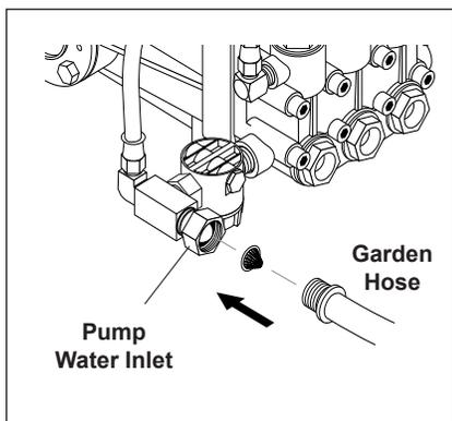
**STEP 7:** Check inlet filters, remove debris, then connect garden hose to pump water inlet.
