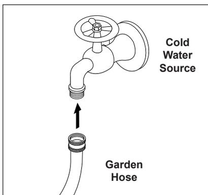
**STEP 3:** Connect garden hose to the cold water source and turn water on completely. Never use hot water.
