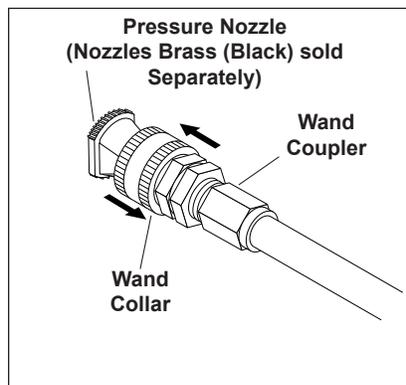
**STEP 3:** Release the coupler collar and push the nozzle until the collar clicks. Pull the nozzle to make sure it is seated properly.
