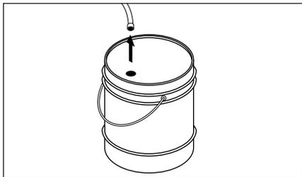
**STEP 1:** Remove detergent suction tube from container and insert into one gallon of fresh water. Slide nozzle forward for low pressure or to connect black detergent nozzle. Pull trigger on spray gun and siphon water for one minute.
