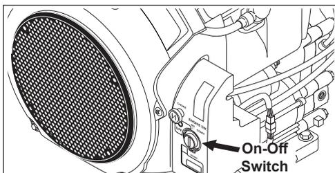
**STEP 2:** Turn engine switch to "OFF" position.
