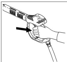
**STEP 4:** With the engine running, pull trigger to operate machine. Liquid detergent is drawn into the machine and mixed with water. Apply detergent to work area. Do not allow detergent to dry on surface.
