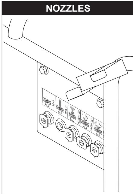
The four color-coded quick connect nozzles provide a wide array of spray widths from 15° to 40° and are easily accessible when placed in the convenient rubber nozzle holder, which is provided on the front of the machine.
