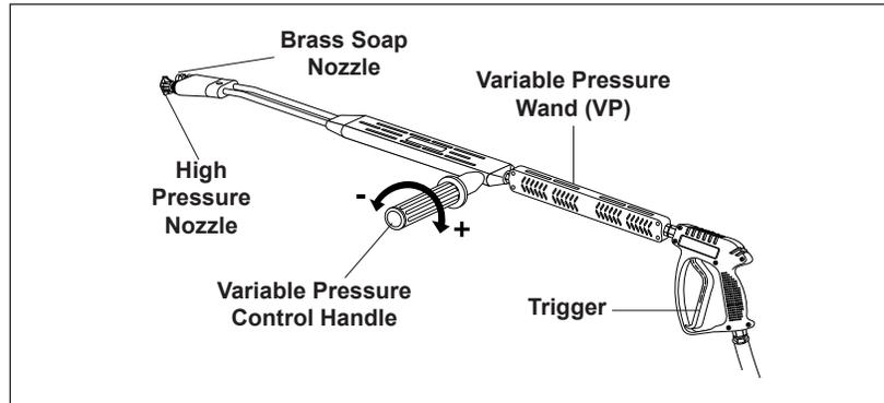
Selection of high or low pressure is accompanied by turning the handle. **Note:** High pressure nozzle must be inserted at end of wand to obtain high pressure. To apply soap read operator's manual.
