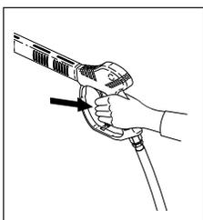
**STEP 4:** Press trigger to release water pressure.
