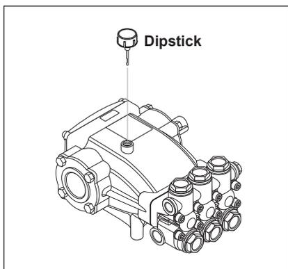
**STEP 4:** Remove shipping cap and install oil dipstick. Check pump oil level by using dipstick or observe oil level in oil window (if equipped). Use 20/40W non detergent oil.
