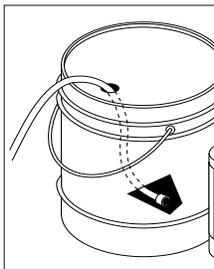
**STEP 2:** Use detergent designed specifically for pressure washers. Household detergents could damage the pump. Prepare detergent solution as required by the manufacturer. Fill a container with pressure washer detergent. Place the filter end of detergent suction tube into the detergent container.
