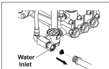
**STEP 5:** Disconnect the garden hose from the water inlet on the machine.
