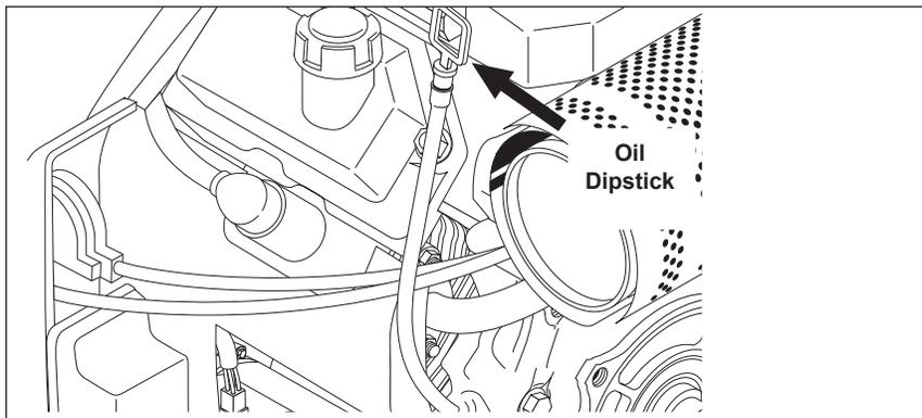
**STEP 1:** Check engine oil level. Oil level should be level with the bottom of the oil filler neck. Be sure the machine is level when checking the oil level. (Refer to the engine's operating manual included with machine.) We recommend that the oil be changed after the first 5 hours of use, then once every 50 hours. **Note:** Improper oil levels will cause low oil sensor to shut off engine. **IMPORTANT! Do not run engine with high or low oil levels as this will cause engine damage.**
