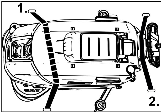
7. First fit the strap under the waste water tank.
