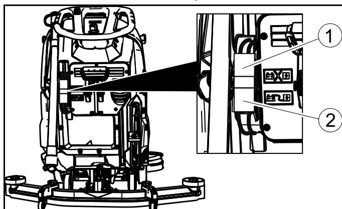
① Battery plug, device side
