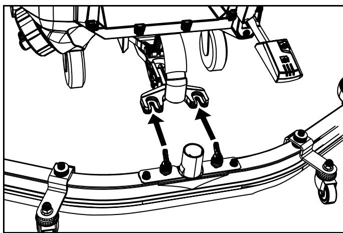
2. Tighten the wing nuts.
