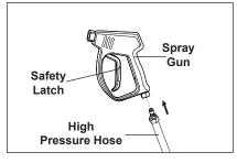
**STEP 1:** Attach the high pressure hose to the spray gun using teflon tape on hose threads.
