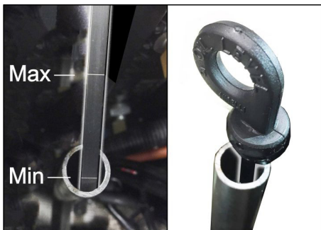
Figure: Measuring the oil level in the petrol motor (KM 105/... and KM 125/...)
