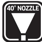
The 40° Nozzle is efficient for general purpose cleaning. Use to remove loose dirt and grime from most surfaces including cars, wood decks, patios, outdoor furniture, home siding and lawn & garden equipment.
