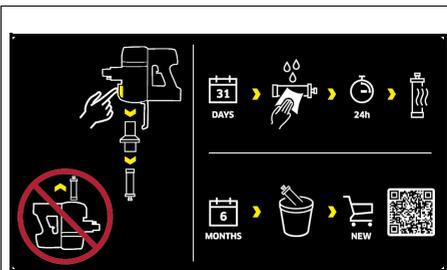
There is a label on the dust container of the device that describes how to clean/replace the cyclone and air inlet filter:
