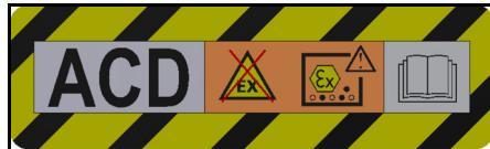
The device is suitable for vacuuming flammable dusts, installation outside zone 22.
