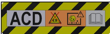
The device is suitable for vacuuming flammable dusts, installation outside zone 22.
