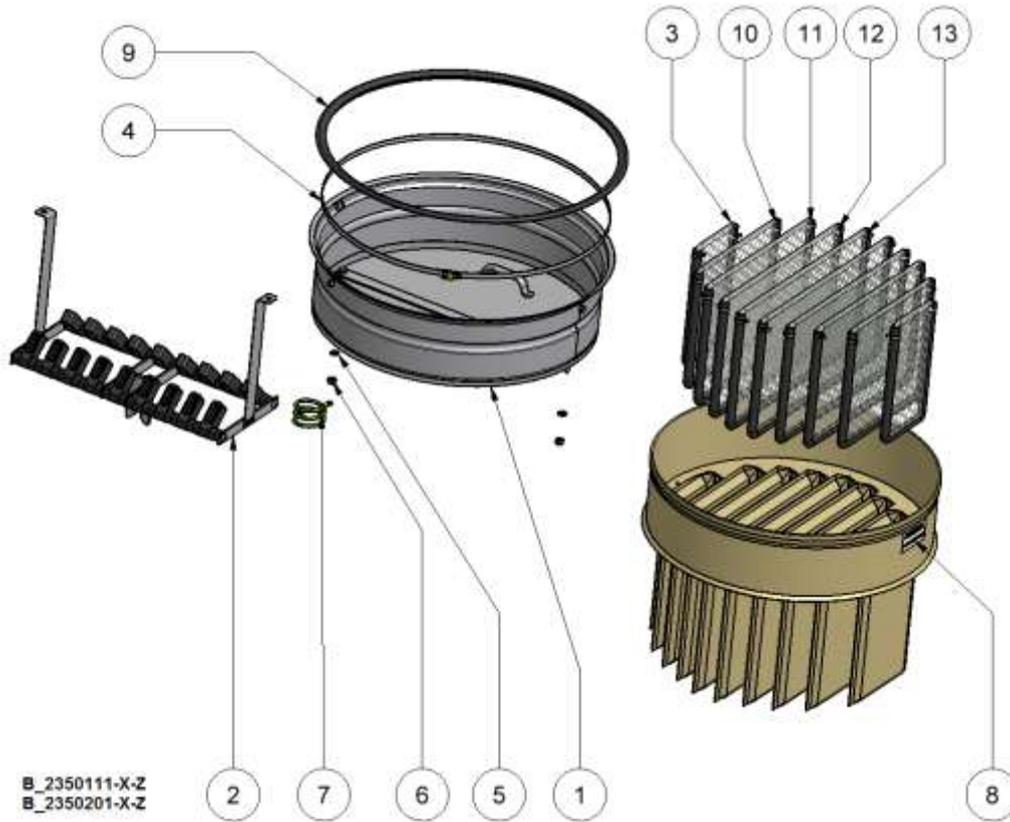
**12.10 Ersatzteilliste/Zeichnung Taschenfilter 1,75m<sup>2</sup>, Kat. "L" as / "M" as (2350201/2350111)**
