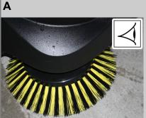
Check the sweeping roller and the side brush for wear and wrapped belts.
