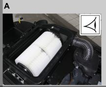
Check dust filter and clean filter box, if required.
