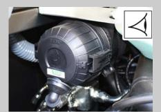
A Check the centrifugal separator and the air filter, clean if required.
