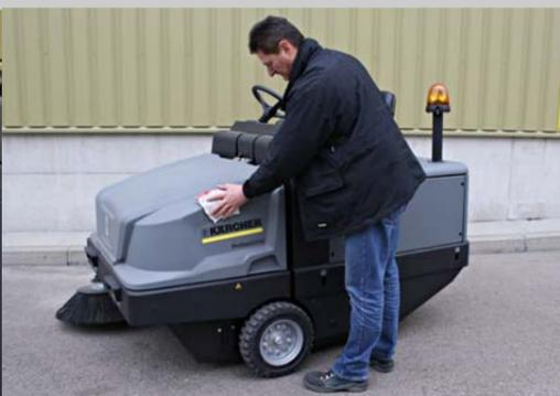
A Check dust filter and clean filter box, if required.
