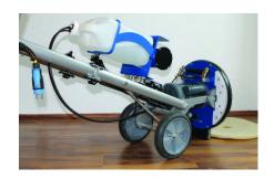
Lift the machine until the wheels slightly come off the ground and push slowly forward until the machine base tilts towards the ground.
