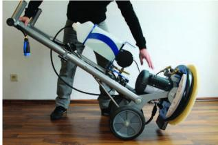
The machine base should now rest on the black bumper foot, located at the back of the bumper. To avoid damage to the handle frame, DO NOT lay the machine frame on the floor as done with other traditional cleaning equipment.
