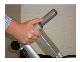
By adjusting the yellow lever you can vary the spray pressure. The further you move the lever counter-clockwise upwards, the higher the water pressure. A horizontal position means maximum water output at maximum pressure.
