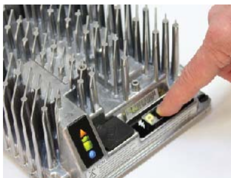
Figure 3: Press the Select Charge Profile Button to advance through the charge profiles. Hold the button for 10 seconds to confirm your selection.
