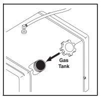
**STEP 2:** Fill gas tank with unleaded gasoline. Do not use leaded gasoline.
