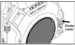
**STEP 5:** Pull the choke lever out to the "Choke" position (on a warm engine, leave the choke lever in the run position). Push the choke lever to the "Closed" position. To restart a warm engine, leave the choke lever in the "Open" position.
