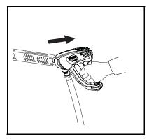
**STEP 4:** Before installing pressure nozzle, trigger spray gun to eliminate trapped pressure. Then run machine, allowing water to flush through the system until clear.
