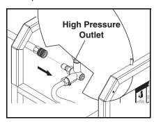
**STEP 7:** Disconnect the high pressure hose from high pressure outlet.
