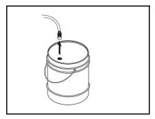
**STEP 1:** Remove detergent suction tube from container and insert into one gallon of fresh water. Open detergent metering valve. Pull trigger on spray gun and siphon water for one minute. Close detergent valve.
