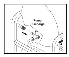
**STEP 4:** Connect the high pressure hose to the pump discharge fitting. Thread twist connect to discharge fitting by turning clockwise.
