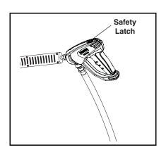
WARNING! Never replace nozzle without engaging the safety latch on the spray gun trigger.
