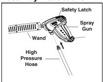
**STEP 1:** Attach wand and hose to the spray gun using teflon tape on threads to prevent leakage.
