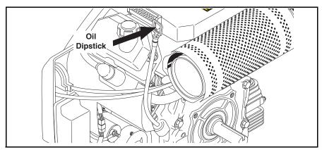
**STEP 1:** Check engine oil level. Oil level should be level to the fill markings on the dipstick. Be sure the machine is level when checking the oil level. (Refer to the engine's operating manual included with machine.) We recommend that the oil be changed after the first 5 hours of use, then once every 100 hours. **NOTE:** Improper oil levels will cause low oil sensor to shut off engine. *IMPORTANT! Do not run engine with high or low oil levels as this will cause engine damage.*
