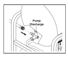
**STEP 4:** Connect the high pressure hose to the pump discharge fitting. Thread twist connect to discharge fitting by turning clockwise.
