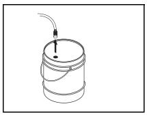
**STEP 1:** Remove detergent suction tube from container and insert into one gallon of fresh water. Open detergent metering valve. Pull trigger on spray gun and siphon water for one minute. Close detergent valve. Turn burner switch off and continue spraying, allowing the water to cool to below 100°F.
