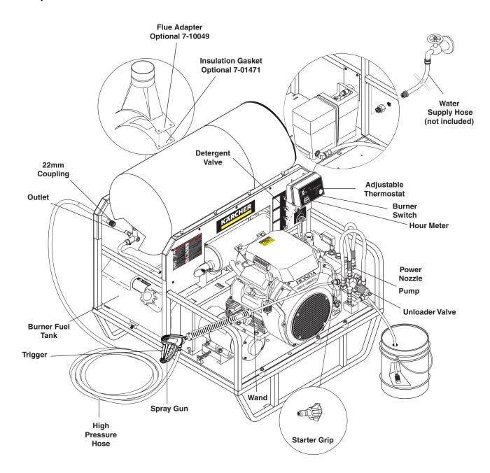
**Pump** — Delivers a specific gpm to the high pressure nozzle which develops pressure.
