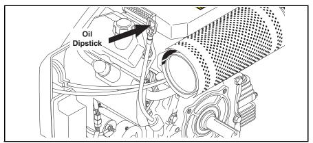
**STEP 1:** Check engine oil level. Oil level should be level to the fill markings on the dipstick. Be sure the machine is level when checking the oil level. (Refer to the engine's operating manual included with machine.) We recommend that the oil be changed after the first 5 hours of use, then once every 100 hours. **NOTE:** Improper oil levels will cause low oil sensor to shut off engine. **IMPORTANT! Do not run engine with high or low oil levels as this will cause engine damage.**
