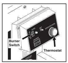
**STEP 9:** Turn the burner switch "ON". Turn thermostat dial to the 210° mark.
