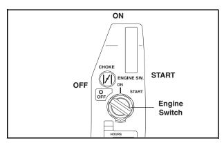
**STEP 8: (Electric Start Models)** Turn the key to the START position, and hold it there until the engine starts. If the engine fails to start within 5 seconds, release the key, and wait at least 10 seconds before operating the starter again.
