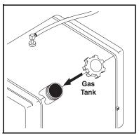
**STEP 2:** Fill gas tank with unleaded gasoline. Do not use leaded gasoline.
