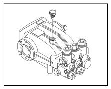
STEP 3: Remove shipping cap and install oil dipstick (Depending on type of shipping, dipstick may already be installed). Check pump oil level by using dipstick or observe oil level in oil window (if equipped). Use SAE 10W-40 weight oil, non-foaming oil.
