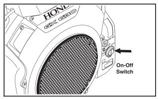
**STEP 7: (Electric Start Models)** Turn the engine switch to "Start" position.
