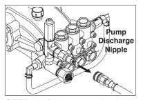
**STEP 6:** Disconnect the high pressure hose from pump discharge nipple.
