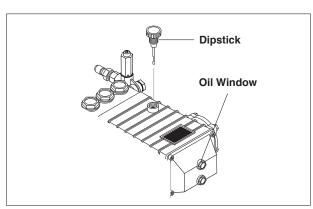
STEP 2: Remove shipping cap and install oil dipstick. Check pump oil level by using dipstick or observe oil level in oil window (if equipped). Use 30 wt. (non detergent) oil.
