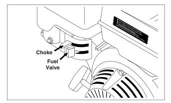
STEP 5: Rotate the fuel shut-off valve to the "On" position. Slide the fuel valve lever to the "ON" position. When the engine is not in use, leave the fuel valve in the "OFF" position.
