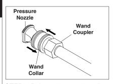
**STEP 7:** Release the coupler collar and push the nozzle until the collar clicks. Pull the nozzle to make sure it is seated properly.
