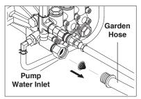
**STEP 5:** Disconnect the garden hose from the water inlet on the machine.
