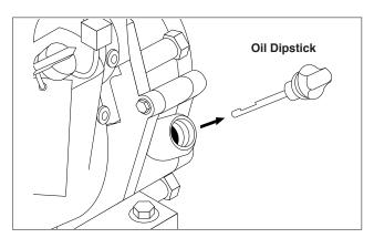
STEP 1: Check engine oil level. Oil level should be level with the bottom of the oil filler neck. Be sure the machine is level when checking the oil level. (Refer to the engine's operating manual included with machine.) We recommend that the oil be changed after the first 5 hours of use, then once every 50 hours. Note: Improper oil levels will cause low oil sensor to shut off engine. IMPORTANT! Do not run engine with high or low oil levels as this will cause engine damage.
