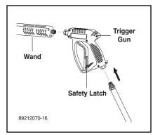
**STEP 3:** Attach variable pressure control wand to spray gun using teflon tape on threads to prevent leakage.
