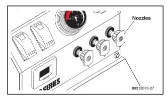
**STEP 6:** The four color-coded quick connect nozzles provide a wide array of spray widths from 15° to 40° and are easily accessible when placed in the convenient rubber nozzle holder, which is provided on the front of the machine. **NOTE:** For a more gentle rinse, select the white 40° nozzle. To scour the surface, select the yellow 15° nozzle.
