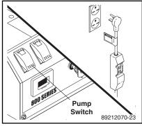
**STEP 2:** Plug unit into power source, push reset button on GFCI, then activate pump switch
