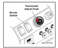
**STEP 4:** For hot water, turn the thermostat knob to 210° then push the burner switch to ON when a steady stream of water flows out of the spray gun. Burner will now light automatically. **NOTE:** Do not start machine with burner switch on.
