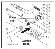
**STEP 1:** Attach a 5/8" water supply hose to inlet connector. Minimum flow should be 5 GPM depending on model of machine. Do not exceed 65 psi incoming water pressure.
