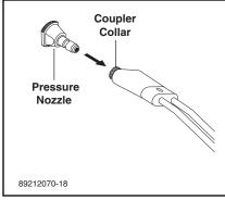
STEP 5: Before installing nozzle, turn on water supply and run machine allowing water to flush through the system until clear. Pull the spring-loaded collar of the wand coupler collar back to insert your choice of pressure nozzle.
