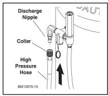
**STEP 2:** Attach high pressure hose to discharge nipple using quick coupler. Lock coupler securely by pulling back coupler collar, inserting onto discharge nipple and pushing collar forward until secure.
