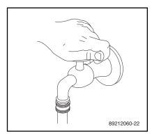
**STEP 1:** Turn on the water. Check for water leaks, tighten as needed.
