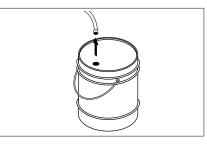
**STEP 1:** Remove detergent suction tube from container and insert into one gallon of fresh water. Slide nozzle forward for low pressure or to connect black detergent nozzle. Pull trigger on spray gun and siphon water for one minute.
