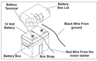
**STEP 8:** Place battery in battery box. Use a 12 V battery with a minimum capacity of 24AH.
