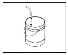
**STEP 1:** Remove detergent suction tube from container and insert into one (1) gallon of fresh water. Pull trigger on spray gun and siphon water for one minute.
