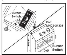
**STEP 5:** For hot water, turn burner switch ON when a steady stream of water flows out of the spray gun. Burner will light automatically.
