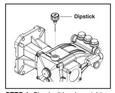
**STEP 4:** Check oil level on sight glass on side of pump. Oil should be visible one-half way up sight glass (SAE 10W-40 non-foaming). The oil level can also be checked by using the dipstick on the top of the pump.
