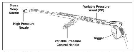
Selection of high or low pressure is accompanied by turning the handle. **NOTE:** High pressure nozzle must be inserted at end of wand to obtain high pressure. To apply soap read Detergents and General Operating Techniques section.
