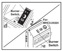
**STEP 2:** Turn burner switch off and continue spraying, allowing the water to cool below 100° F.
