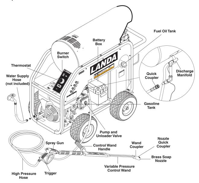
**Pump** — Delivers a specific gpm to the high pressure nozzle which develops pressure.
