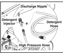
**STEP 2:** Attach high pressure hose to discharge nipple using quick coupler. Lock coupler securely into place by pulling back coupler collar and inserting it onto discharge nipple, then pushing collar forward to lock in place.
