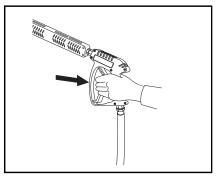
**STEP 4:** With spray nozzle pointed away from you or anyone else, press trigger on spray gun to obtain pressurized cold water spray.
