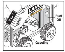
**STEP 5:** Fill gasoline tank and check engine oil. Fill fuel tank. Do not confuse gasoline and fuel oil (diesel) tanks. Keep proper fuel in proper tanks.
