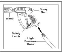
STEP 3: Attach wand to spray gun using teflon tape on threads to prevent leakage. Attach swivel connector on discharge hose to spray gun using teflon tape on threads. Attach swivel connector on high pressure hose to spray gun using teflon tape on threads. Engage safety latch to prevent from triggering gun.
