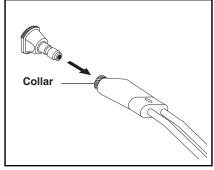
**STEP 2:** Before installing nozzle, turn on water supply and run machine allowing water to flush through the system until clear. Pull wand coupler collar back and insert desired pressure nozzle into coupler then secure by pushing coupler collar forward.
