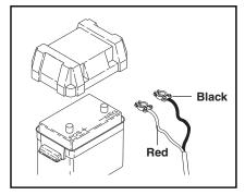
**STEP 6:** On electric start models only, you will need to install a battery making sure that the red cable is attached to the positive terminal. Use a Group U1 garden tractor style type of battery rated for 300 CCA (battery not included).
