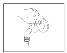
**STEP 1:** Turn on water at faucet and pull trigger on spray gun allowing water to flow until all air has discharged from system. Check for water leaks; tighten as needed.
