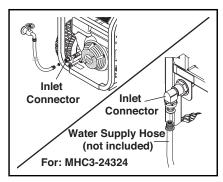
**STEP 1:** Attach a 3/4" garden hose to inlet connector. Minimum flow should be 5 gpm.
