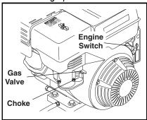
**STEP 3:** Read engine manual, turn on gas valve and choke. Turn the engine switch to the START position and hold it there until the engine starts.
