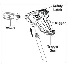
**STEP 5:** Attach variable pressure control wand to spray gun using teflon tape on threads to prevent leakage. Position safety latch to prevent trigger from being pulled.
