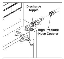
STEP 1: Connect the high pressure hose quick coupler to the discharge nipple by sliding the quick coupler collar back and inserting the quick coupler onto the discharge nipple and pushing the quick coupler collar forward to secure it. Secure desired pressure nozzle into variable pressure wand coupler.
