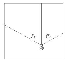
**STEP 1:** Place machine in a convenient location providing ample support, drainage and room for maintenance. Remove pallet bolts and remove pallet, then re-install bolts to level machine by adjusting (machine must be level).
