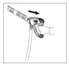
**STEP 3:** Open spray gun to relieve remaining pressure and remove water supply hose.
