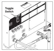
**STEP 3:** Place toggle switch in the ON position and then pull the trigger on the spray gun to activate a pressure switch which will then start the machine. The ON position is for auto shut down.
