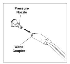
**STEP 6:** Pull the spring-loaded collar of the wand coupler collar back to insert your choice of pressure nozzle.
