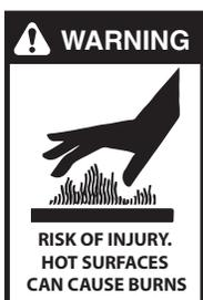
**WARNING:** Risk of injury. Hot surfaces can cause burns. Use only designated gripping areas of spray gun and wand. Do not place hands or feet on non-insulated areas of the pressure washer.
