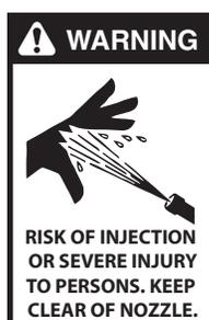
**WARNING:** High pressure developed by these machines will cause personal injury or equipment damage. Keep clear of nozzle. Use caution when operating. Do not direct discharge stream at people or animals, or severe injury or death will result.
