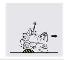
On our ride-on sweepers in the 105/125 model series the sweeping roller is at the rear axle. This means that you always safely ride over obstacles, ramps and barriers. The sweeping system is located between the wheels and follows the wheels at crossings. At the same time, you have perfect accessibility when you need to check or change the sweeper brush. This is very useful, for example, for wrapped up tapes or films.
