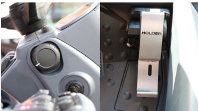
Engine speed can be preselected digitally with memory function/
