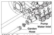
**STEP 7:** Check inlets filters, remove debris, then connect the garden hose to pump water inlet. *CAUTION: Do not run the pump without water or pump damage will result.*
