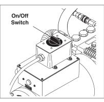
**STEP 4:** Turn machine on by turning switch at top of motor.
