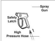
**STEP 1:** Attach the high pressure hose to the spray gun using teflon tape on hose threads.
