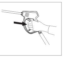
**STEP 2:** Trigger the spray gun to eliminate trapped air then wait for a steady flow of water to emerge from the spray nozzle.
