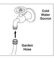
**STEP 1:** Connect garden hose to the cold water source and turn water on completely. Never use hot water.
