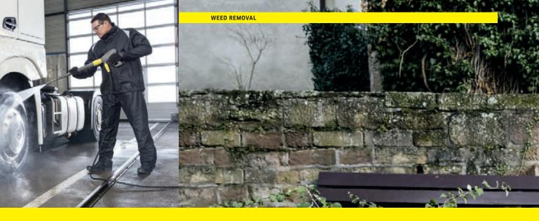
Hot water high-pressure cleaners can increase the water **Cleaning with hot water therefore offers various** inlet temperature from approx. 12 °C to up to 155 °C. This possibilities for optimising the cleaning process using allows for a reduction in the working pressure, the time **the advantages of HDS:** required and the volume of cleaning agent that is used.
