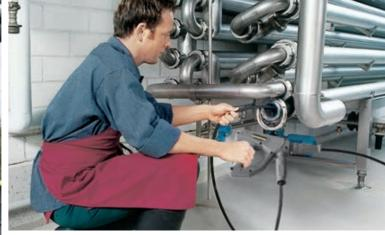
Special accessories for pipe cleaning Clean dirty or blocked drains and pipes in no time. The nozzle openings, which point to the rear, automatically pull the hose into the pipe. Even stubborn deposits of dirt are reliably loosened and washed out of the pipe with the flow of water. Our particularly powerful pipe cleaning dirt blasters use their forward-facing rotating point jet to reliably work through the most stubborn blockages.
