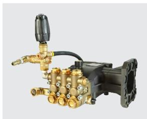
Quick change pump assemblies include a pump, unloader, thermal protector, by-pass loop hose, garden hose inlet with filter, and quick connect coupler. They are easy to install, less expensive than separate components and labor to assemble components, and eliminate the guesswork on selecting components to go with the pump.
