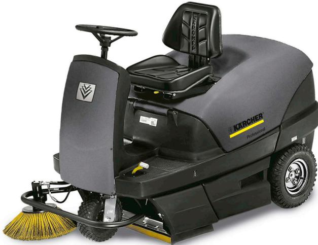
A KM 100/100 R Bp excels in locations where fine dust control is important. A large cylindrical filter effectively contains the toughest dust imaginable. Variable speed in forward and reverse, up-front seating for safety around ends of aisles make this a perfect warehouse sweeper that fits easily into most sweeping budgets. For indoor and outdoor use.
