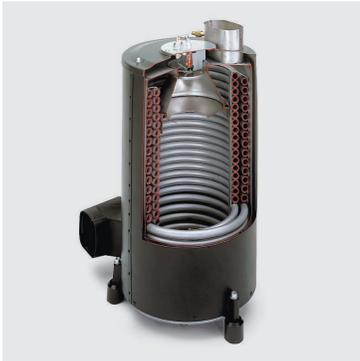
Kärcher's proprietary heating coil is unequalled in the industry for its high heating performance, compact design, and super-efficiency. Double-wall construction – with air passing between the two walls – provides insulation as well as oxygen for the combustion process.
