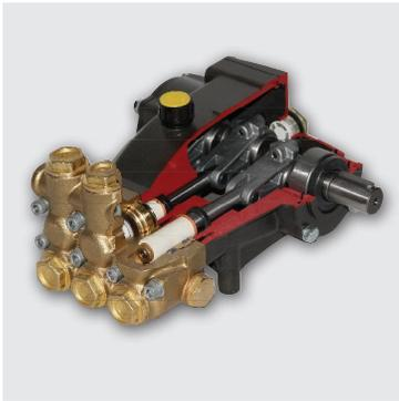
The U-Seals provide better run-dry protection, extend pump life, and allow for inlet water of up to 185°F. Kärcher K3 pumps provide a stronger crankcase with thicker mounting feet and extra-large European made tapered roller bearings for longer pump life. The crankcase is reinforced and comes with the new O-ring seal for leak-free operation. Specially die cast connecting rods provide for quieter operation and longer pump life.
