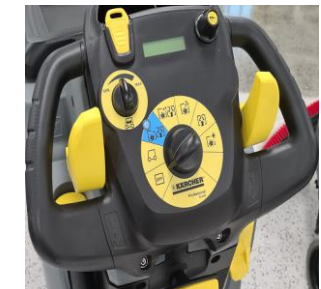
Step 21 Briefly drive forward to suck up the remaining water
