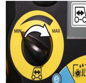
Step 12 Select the driving speed at the rotary knob
