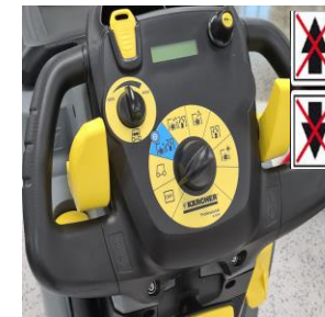
Step 19 Release driving lever
