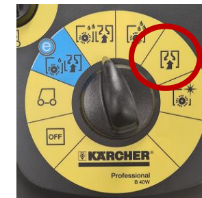
Step 20 Set the program selection switch to suction or vacuum
