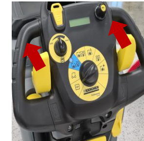
Step 13 To drive forward, press the driving lever to the front. To stop the machine, release the driving lever
