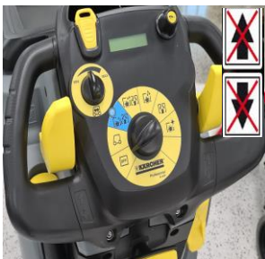
Step 15 To stop, release the driving lever
