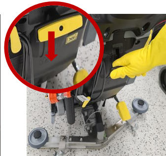
Step 10 Lower the squeegee with the central yellow handle
