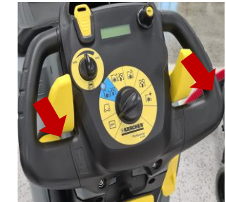
Step 14 To drive reverse, press the driving lever to the rear. To stop the machine, release the driving lever
