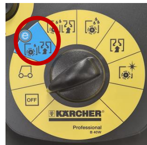
Step 17 For daily cleaning, turn the programme selector switch to Eco mode. You can select other modes if the floor requires
