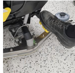
Step 11 Press the pedal for lowering the cleaning head downwards slightly and then move it to the left
