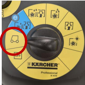
Step 9 Turn the programme selector switch to position 1 "Transport mode"
