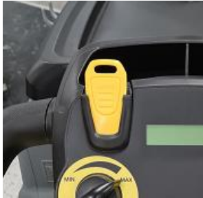
Step 8 Plug in the Intelligent Key
