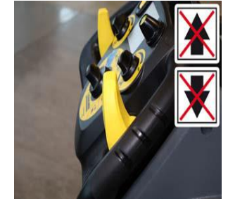
Step 14 To stop, release the driving lever
