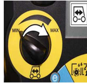
Step 11 Select the driving speed at the rotary knob
