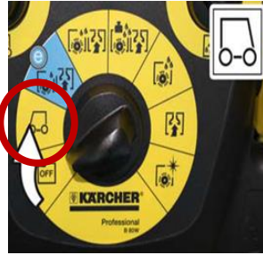
Step 9 Turn the programme selector switch to position 1 "Transport mode"
