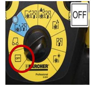
Step 21 Turn the program selection switch to "OFF"
