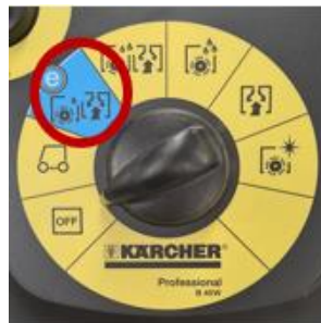
Step 16 For Daily Cleaning, turn the selection switch to Eco mode. You can select other modes if the floor requires it
