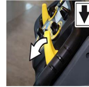
Step 13 To drive in reverse, press the driving lever to the rear. To stop the machine, release the driving lever
