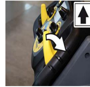
Step 12 To drive forward, press the driving lever to the front. To stop the machine, release the driving lever
