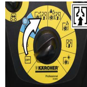
Step 19 Set the program selection switch to suction or vacuum
