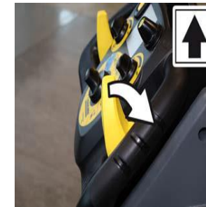
Step 20 Briefly drive forward to suck up the remaining water
