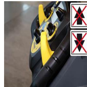
Step 18 Release driving lever
